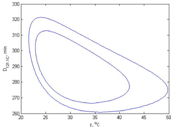
Fig. 9. Case 3. Nasri et al. (1993) data. 95% (inner) and 99% (outer) joint confidence region for parameters  $D_{121,1^{\circ}\text{C}}$  and  $z$  ( $T_r = 376$  K). All points represent constant sum-of-squares of errors per Eq. (26). Computed iteratively per Motulsky and Christopoulos (2004).
