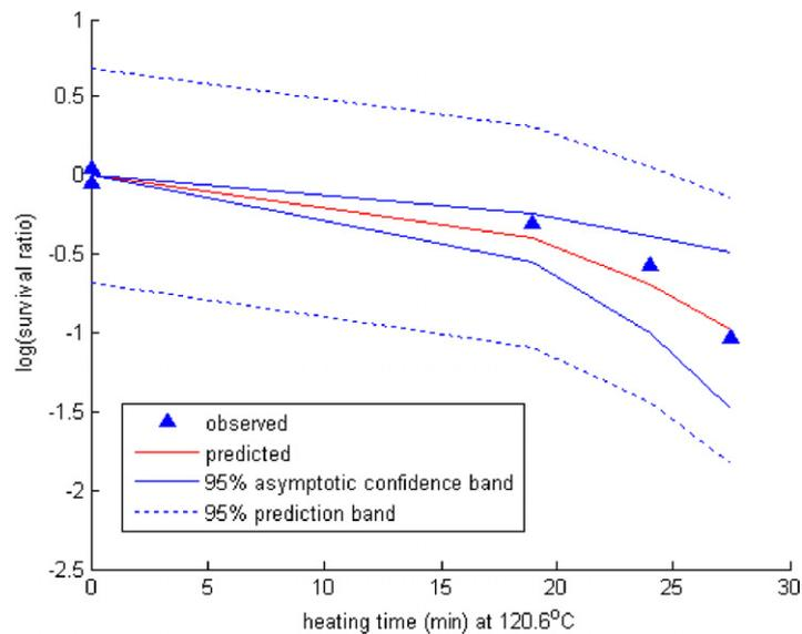
Fig. 8. Case 2. Welt (1996) data. 95% asymptotic confidence band and 95% prediction band for log(survival ratio) for cans heated at retort temperature of 120.6 °C.
