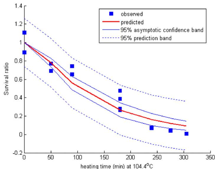
Fig. 2. Case 1. Welt (1996) data. 95% asymptotic confidence band and 95% prediction band for survival ratio for cans heated at retort temperature of  $104.4^{\circ}\text{C}$ . Prediction curve, confidence band, and prediction bands were constructed by minimizing total sum-of-squares for the data in Figs. 2–4.
