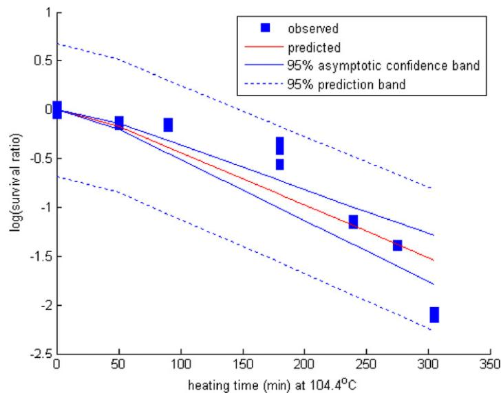
Fig. 6. Case 2. Welt (1996) data. 95% asymptotic confidence band and 95% prediction band for  $\log(\text{survival ratio})$  for cans heated at retort temperature of  $104.4^{\circ}\text{C}$ . Prediction curve, confidence band, and prediction bands were constructed by minimizing total sum-of-squares for the data in Figs. 6–8.
