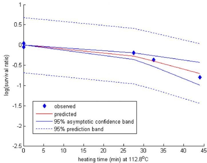
Fig. 7. Case 2. Welt (1996) data. 95% asymptotic confidence band and 95% prediction band for log(survival ratio) for cans heated at retort temperature of 112.8 °C.
