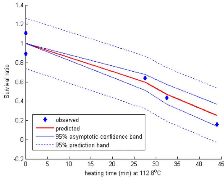
Fig. 3. Case 1. Welt (1996) data. 95% asymptotic confidence band and 95% prediction band for survival ratio for cans heated at retort temperature of 112.8 °C.
