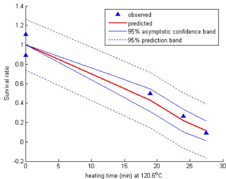
Fig. 4. Case 1. Welt (1996) data. 95% asymptotic confidence band and 95% prediction band for cans heated at retort temperature of 120.6 °C.
